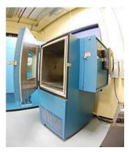
Environmental chamber to simulate temperatures and humidities encountered by packages
