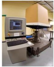
Vibration tester to simulate vibration frequencies at which packaged products are subjected during shipments
