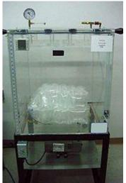
Vacuum chamber for testing leaks in packaging component
