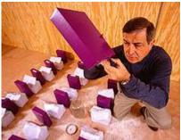
Testing the ability of packages to resist insect infestation
