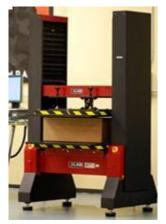
Packaging compression tester to determine the stacking strength of packaging
