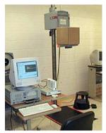
Instrumented drop test of cushioned package to measure the transmitted shock
