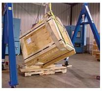
Rotational corner drop test of wooden box
