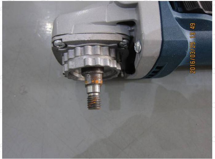
Found rust mark
