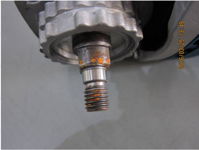
Details of rust mark
